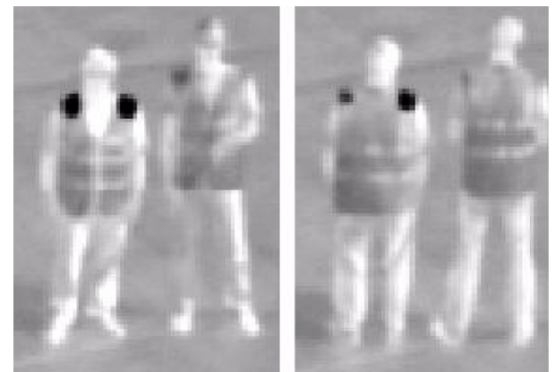
Figure 4. IR T (8-12 \mu m) images of subjects wearing Mirage TM -marked (left) and unmarked (right) high-visibility jackets.
