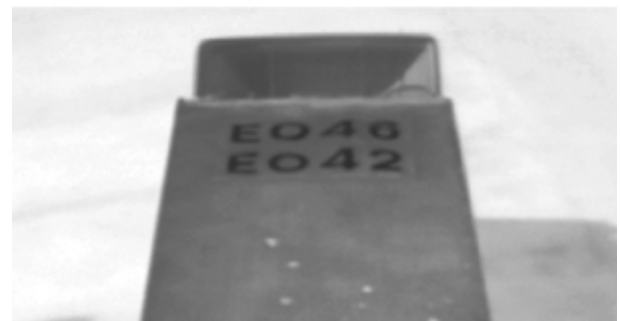
Figure 3. Visible and IR T (8-12 \mu m) images of a heavy goods vehicle marked with 360mm high TransportHeavy font letters and numbers cut from Mirage TM vehicle marking film on a conventional white vinyl background.
