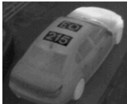
Figure 1. Visible and IR T images (3-5 \mu\text{m} ) of a vehicle marked with the new Mirage TM material.
